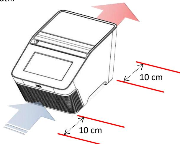
Please make sure there is no obstacle in the air flow path. At least 10 cm of space is required at the front and the back of the instrument.
